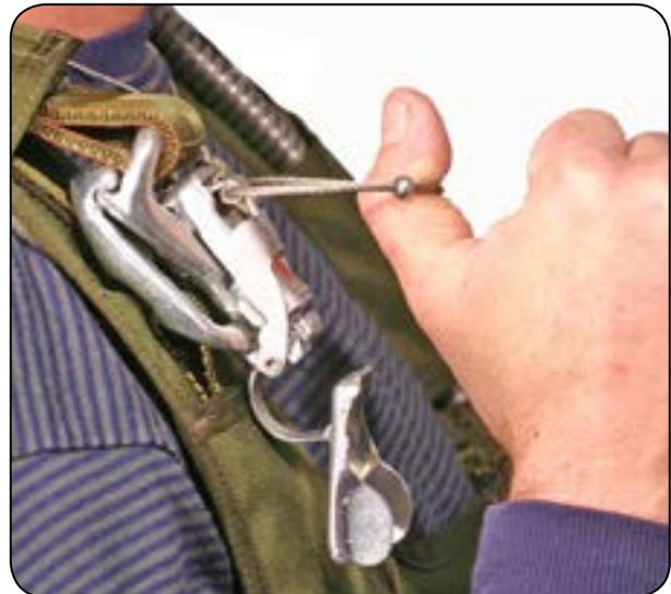
Pull the cable loop until the canopy riser releases.
