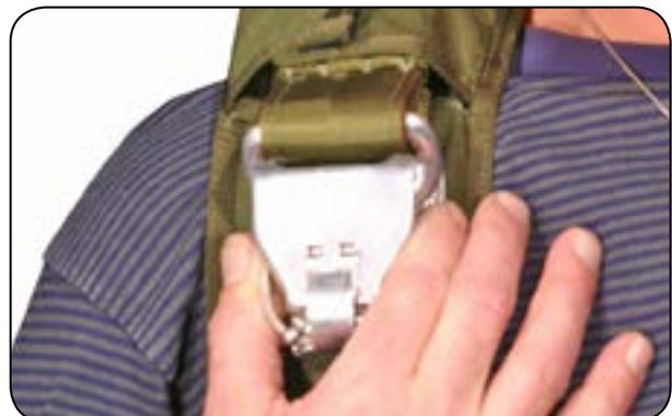
Pull the cover out and down to expose the cable loop.
