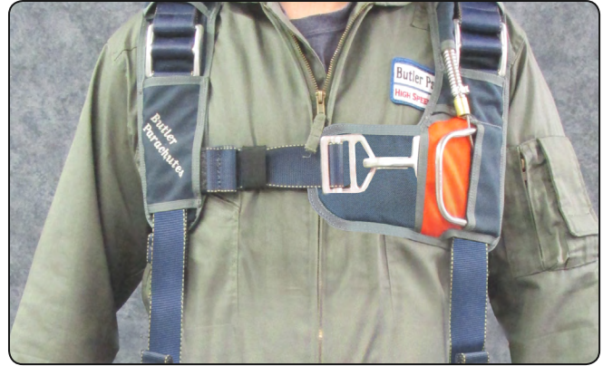
6.1 Attaching the chest strap.
