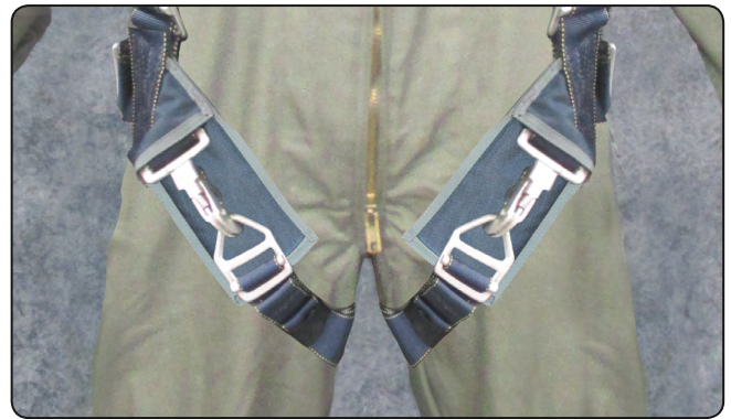
6.2 Attaching the leg straps.
