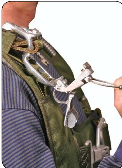
Pull the cable loop until the canopy riser releases.
