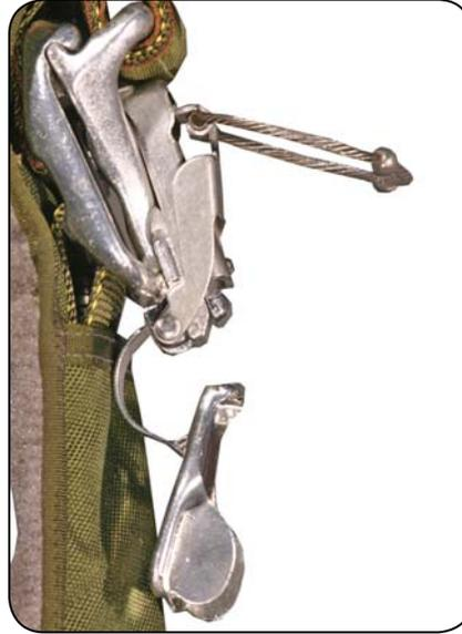
Pull the cover out and down to expose the cable loop.
