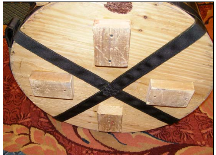
Longitudinal (Vertical) cross strap installed on barrel.
