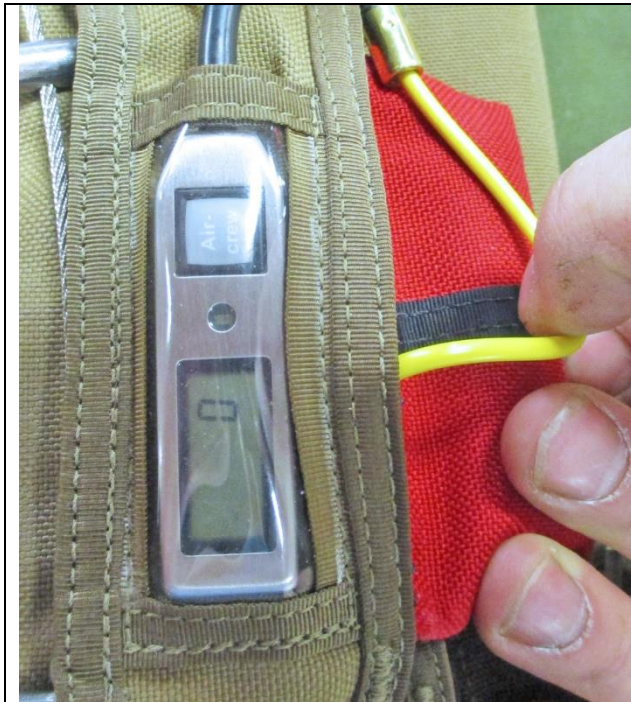
Cable pulled at handle until the Control Unit displays "0"
