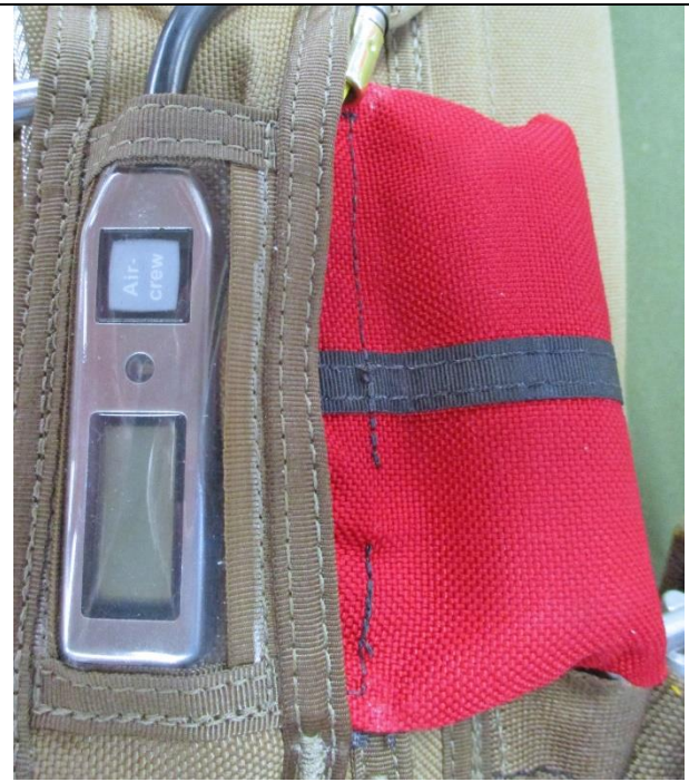
Cable installed – A blank Control Unit means Proper Functionality. If "0" continues to show the unit is defective.
