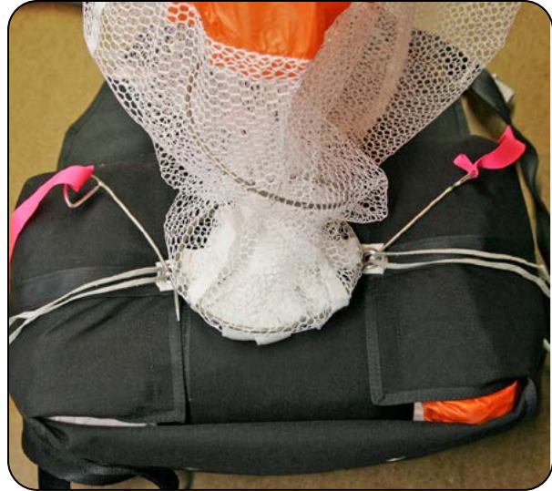
9.12 Stowing the pilot chute.
