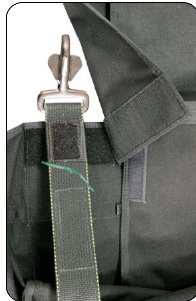
7.1.1 Tacking the riser to the pack tray.
