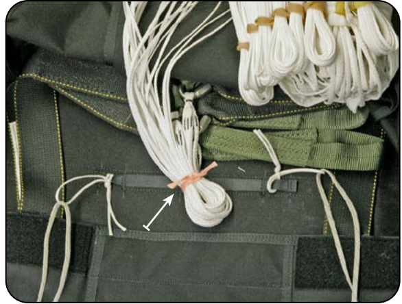
9.3 Forming the break-tie stow.
