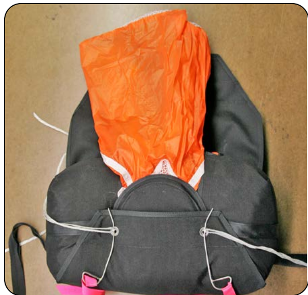
9.16 Closing the bottom flap.
