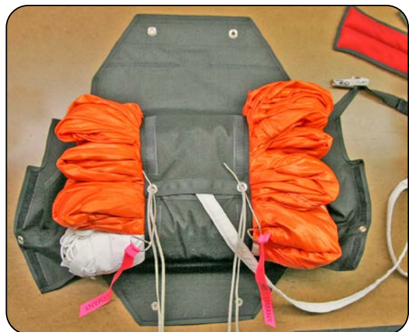
9.8 Closing the top staging flap.
