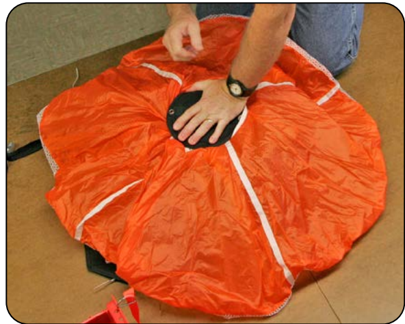
9.13 Compressing the pilot chute.
