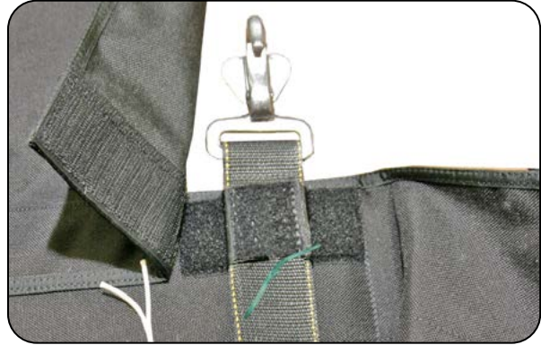
7.2.1 Tacking the riser to the pack tray.
