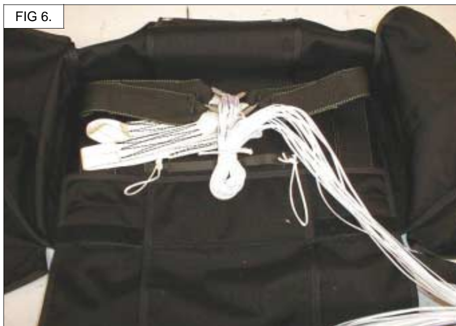
Figure 6. Form a bight in the suspension lines and using the 80lb tape, secure it to the pack tray with a surgeon's and locking knot. Trim the ends to 1 inch. Note: This suspension line tie helps ensure proper staging of the deployment sequence and must be installed.
