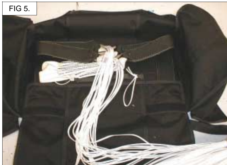
Figure 5. Neatly fold the risers and the cross-connectors across the bottom of the container.
