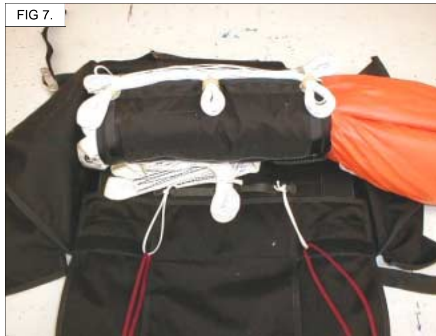
Figure 7. Place the diaper across the bottom of the container on top of the risers and cross-connectors as shown.
