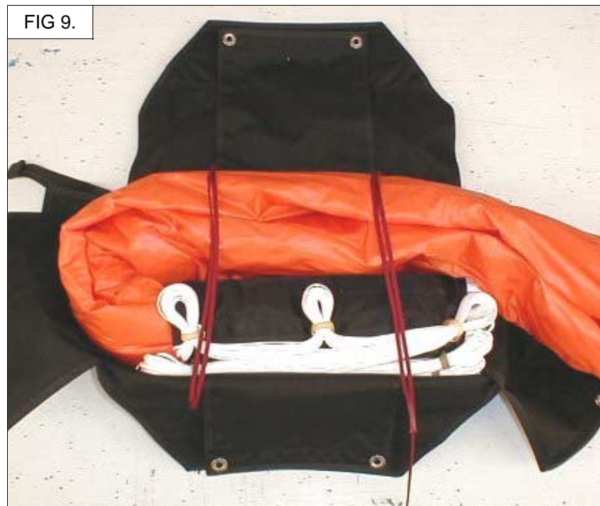
Figure 9. For this size of container, the rigger determined that the diaper plus one fold of the canopy is the correct amount to place between the closing loops and the bottom of the container.
