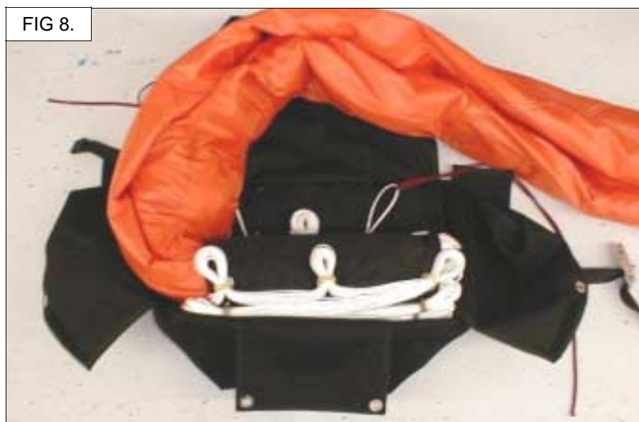
Figure 8. Rotate the container as needed to begin “S” folding the canopy into it. Depending on the container size, the amount of canopy “S” folded between the closing loops and the inner staging flaps will vary and is up to riggers discretion.
