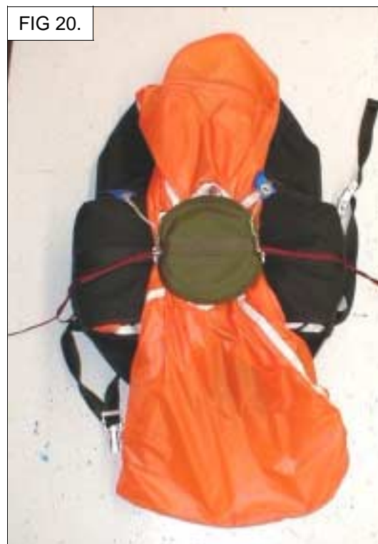
Figure 20. Overhead view of pilot chute compressed and pinned in place.
