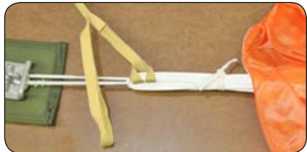
7.2 Installing the zip-strip to the apex.
