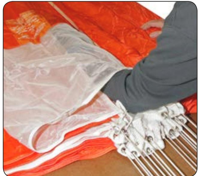
\* THE LOPO SERIES DOES NOT HAVE A STOP RING. SEAT THE GROMMET AGAINST THE CANOPY SKIRT.
