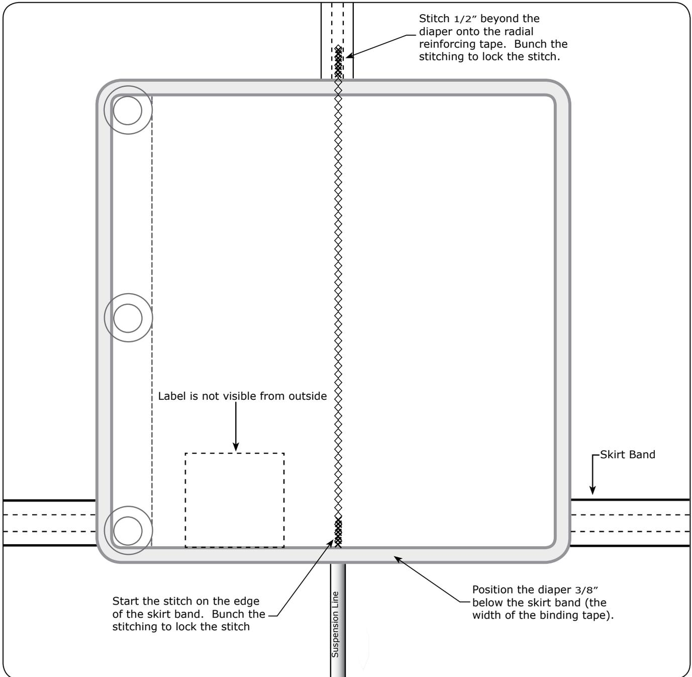
Install the diaper on the outside of the front radial seam with the bottom edge of the diaper 3/8" (width of the binding tape) below the bottom of the skirt band.
