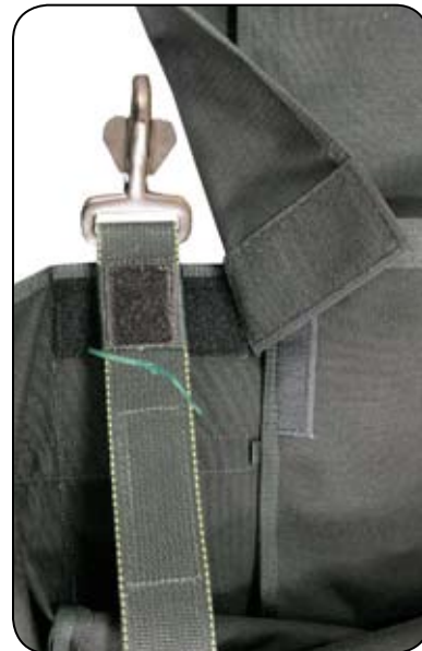
7.1.1 Tacking the riser to the pack tray.
