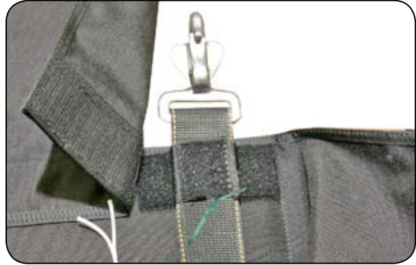
7.2.1 Tacking the riser to the pack tray.
