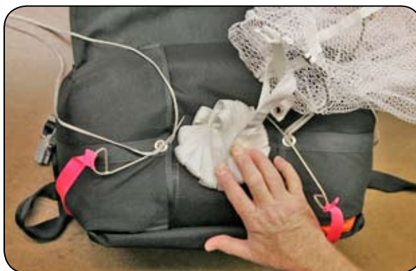
9.11 Folding the pilot chute bridle.
