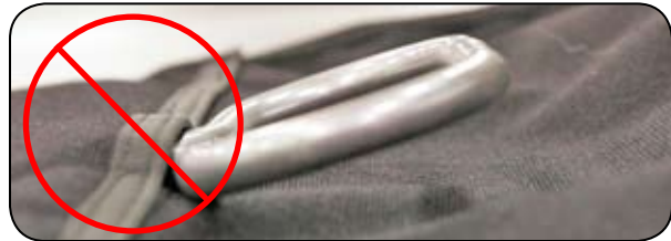
WRONG RIPCORD PLACEMENT.
