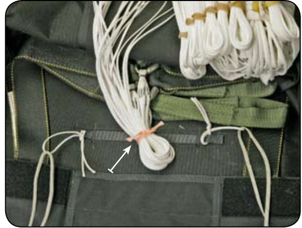
9.3 Forming the break-tie stow.
