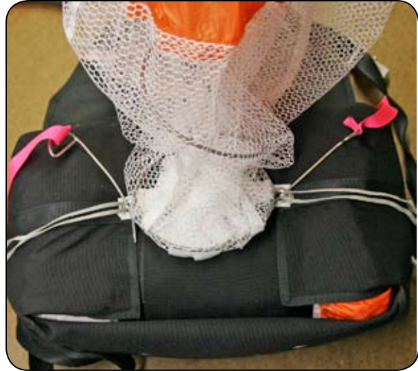
9.12 Stowing the pilot chute.
