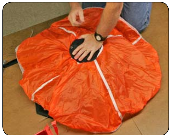
9.13 Compressing the pilot chute.
