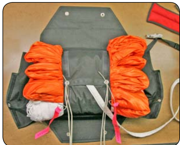
9.8 Closing the top staging flap.
