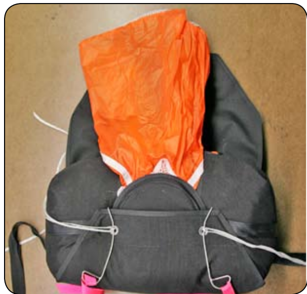
9.16 Closing the bottom flap.
