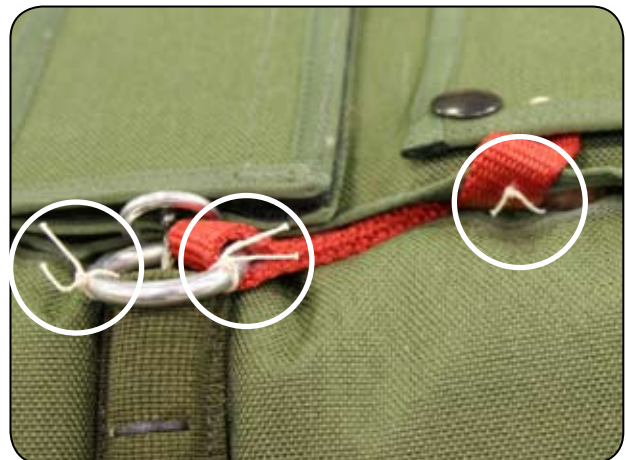
6.4 Tacking the finished installation.
