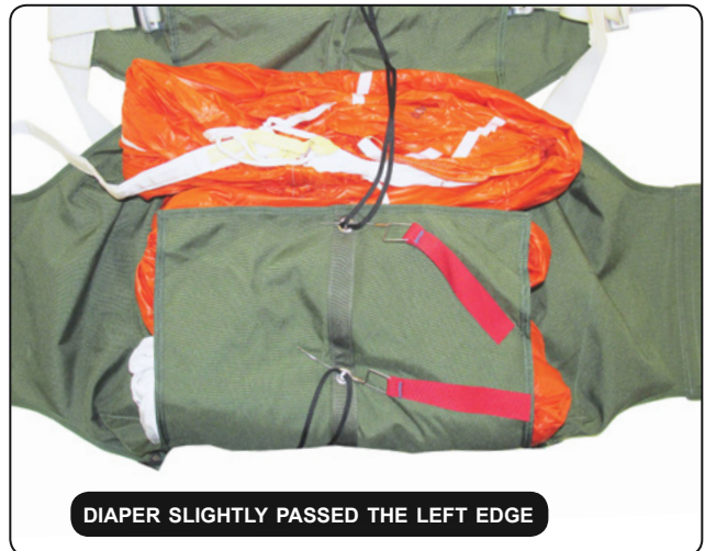
7.11 Closing the bottom flap.
