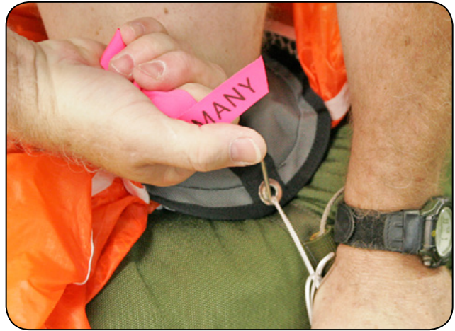
7.19 Pinning the pilot chute.
