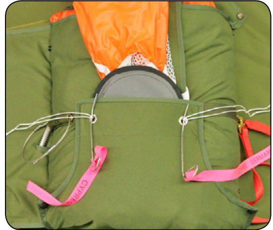
7.22 Closing the left container flap.
