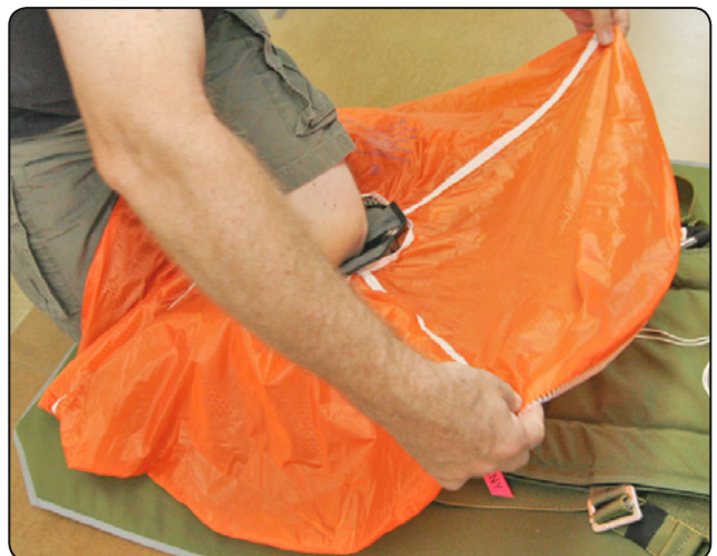
7.15 Compressing the pilot chute.
