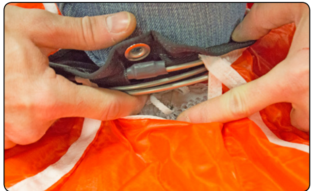
7.17 Folding and stowing the center line.
