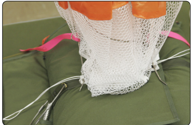
7.14 Setting the pilot chute.
