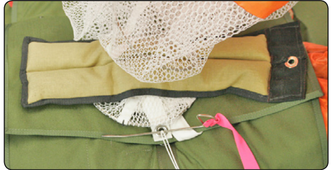
7.13 Stowing the pilot chute bridle.
