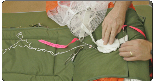
7.13 Stowing the pilot chute bridle.
