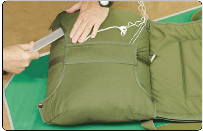
7.25 Dressing the container.
