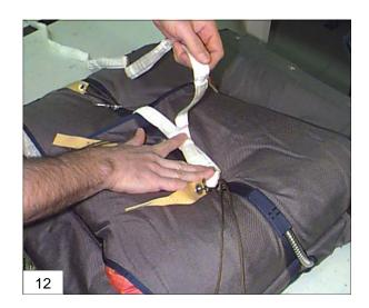
13. Position the pilot chute base on top of the folded, pilot chute bridle, aligning the grommets located on the base of the pilot chute with the top flap grommets. Pass your pull-up cord through the bottom pilot chute grommet and pin the pilot chute in place.
