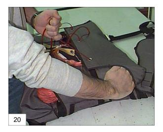
21. Repeat the closing procedure with the closing loop on the opposite end. Again, use a packing paddle to smooth any wrinkles.
