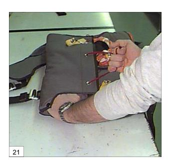
22. After pinning the top closing loop, pull up on the center closing loop and pin; again taking care to keep the inner flaps in postion and to keep the pack nice and flat.
