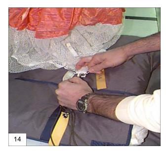
14. Pass the center pull-up cord through the bottom pilot chute grommet and pin in place.
