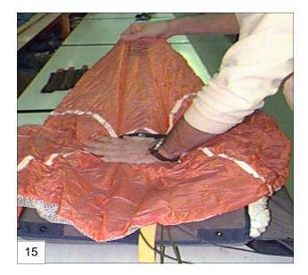
16. Hold the compressed pilot chute in place (your knee works well). Carefully fold the pilot chute material that is covering the bottom of the container and place it against the compressed pilot chute. DO NOT TRAP ANY MATERIAL INSIDE THE PILOT CHUTE SPRING! Pass your pull-up cord through the grommet on the pilot chute crown and pin.
