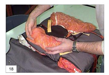
19. Tuck the folded pilot chute material around the pilot chute crown taking care to support the spring as noted previously.
