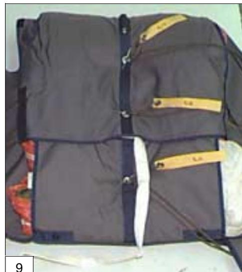
10. Mate the 6” sections of Velcro on the sides of the top flap by pulling the top flap over, down and around the canopy and fastening it to the corresponding Velcro on the pack tray. Leave some of the canopy material sticking out on all four corners – doing so will fill the corners of the container and result in a cleaner looking container when closed. Be sure to keep the bottom flap in position during this procedure.
