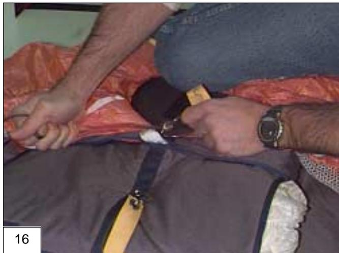
17. As in the previous step, fold the pilot chute material covering the top of the container, and pin the pilot chute crown in place.
