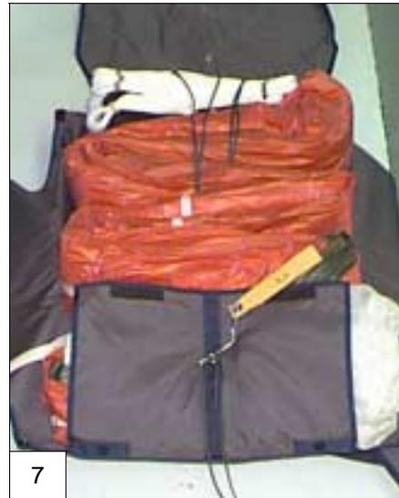
8. Pass the top and center pull-up cords through the grommets in the top flap, fold the flap over the canopy, and hold in place with temporary pins. The top flap will overlap the bottom flap approximately 1”.
