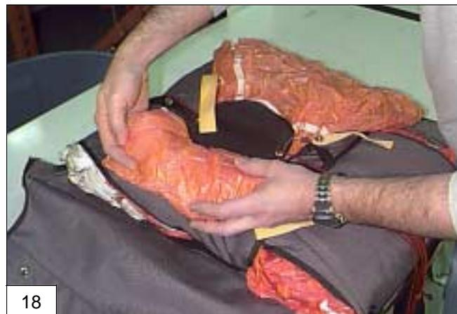
19. Tuck the folded pilot chute material around the pilot chute crown taking care to support the spring as noted previously.
