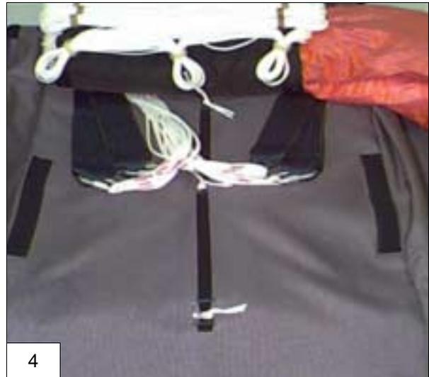
5. Pass one end of a 12 inch piece of 80 lb. cotton tape under the Type IV webbing adjacent to the center pack closing loop. Form a bight in the suspension lines and using the 80 lb. tape, secure it to the closing loop attachment tape with a surgeon's and locking knot. Take care to ensure that the location of this bight does not end up underneath the pilot chute spring. Trim the ends to 1 inch of the knot.
