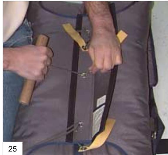
26. Keeping the corners as neat and full as possible, carefully close the corners of the containers as shown. Use your finger to reach inside and poke the corner tuck out if needed.
