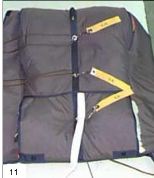
12. “S” fold the pilot chute bridle between the top and center grommets on the top flap.
