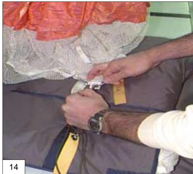
15. Compress the pilot chute and pull all of the material clear of the spring.
