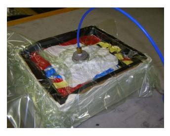
A2-5) The parachute is sucked down to the rigger's satisfaction and is ready to go into the oven to bake.
