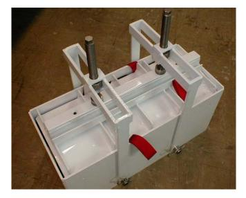
A1-5) Packing fixture with parachute compressed to proper point to soak and relax.
