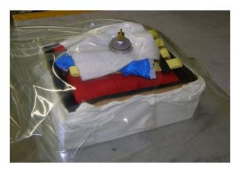
A2-3) The fixture and parachute are "bagged".
