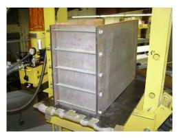
A3-4/5/6) The shell is placed into the fixture, the side and end plates are closed up, then tightened down with the cross bolts.
