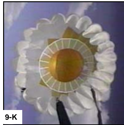
Butler Parachute HX-500 test drop. 180 KIAS @ 528 lb. On-board camera showing close-up of inflation process.
