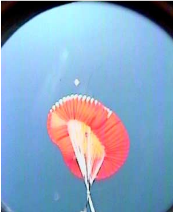
Figure 15: Main parachute approaching reefed inflation.
