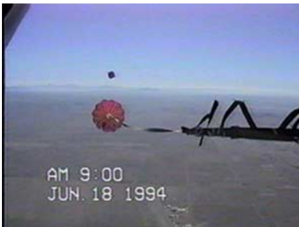
Figure 11: The extraction parachute just after inflation.
