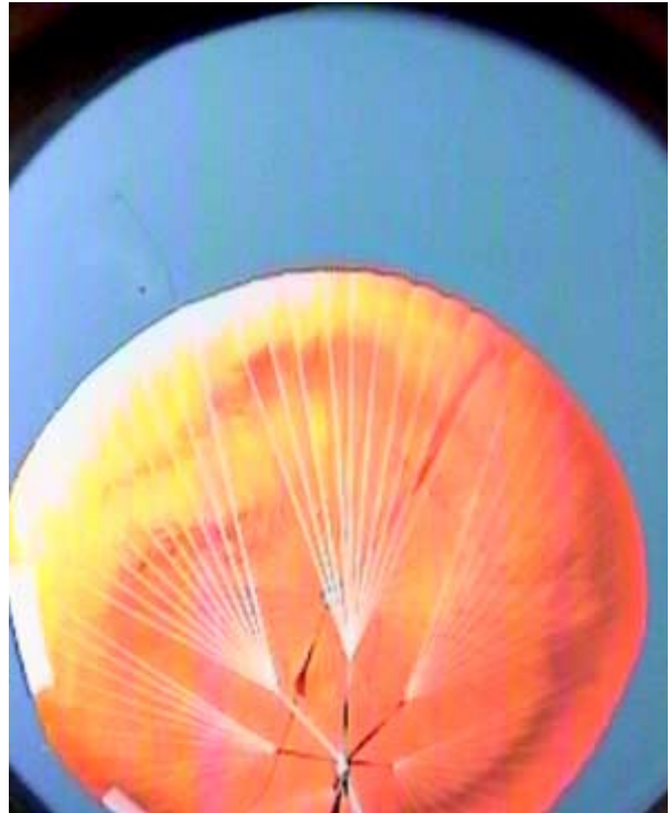
Figure 16: Main parachute at full inflation.
