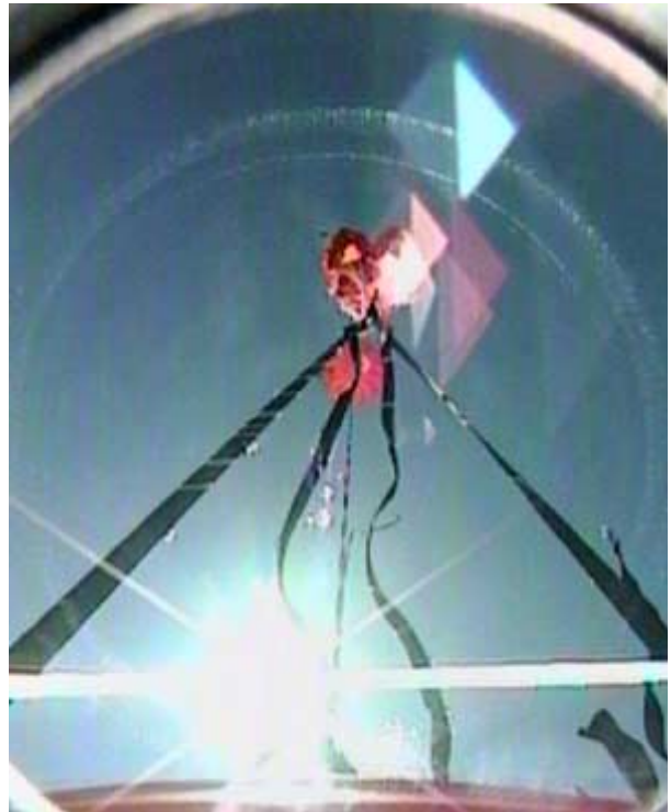
Figure 14: Main parachute just after extraction from the quarter bag.
