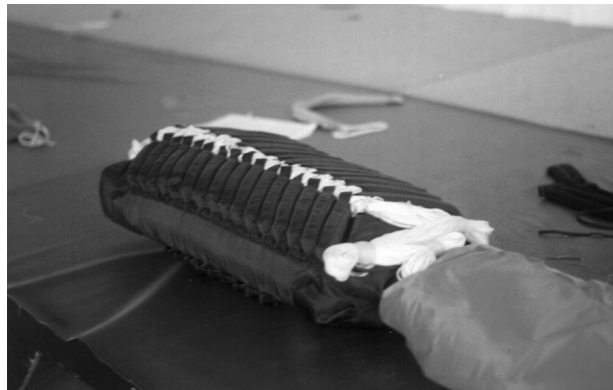
Figure 7: The packed quarter bag.
