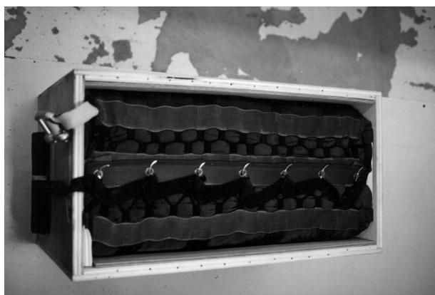
Figure 8: The packed recovery system in its transfer container.
