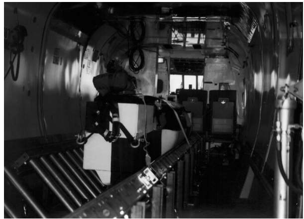
Figure 10: The air drop test vehicle installed on the aircraft roller track, just before takeoff.
