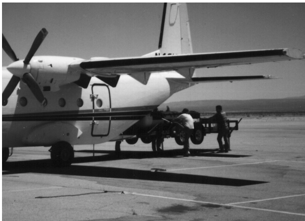
Figure 9: Loading the test vehicle into the aircraft. The trailer has been raised on its jacks to the level of the V-track roller in the aircraft.
