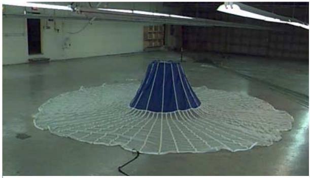
**Photo 1**. Fully extended slider for a G12 canopy. There is a grommet for each line.
