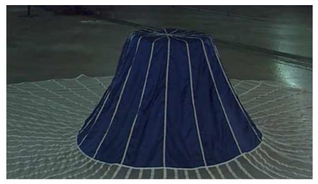
**Photo 2.** Close-up of the hemisphere illustrating that this particular slider has four radials for each gore in the hemisphere and mesh skirt. BPS typically uses two radials up to about 40' diameter canopies.
