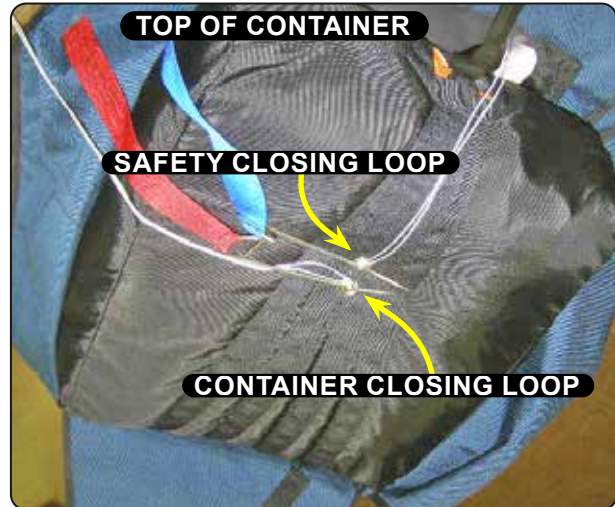
14.3 Pinning the closing loops.
