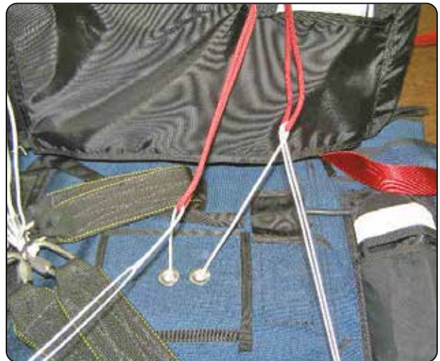
14.2 Threading the closing loops.
