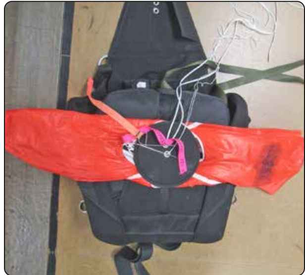
14.16 Pinning the container closing loop.
