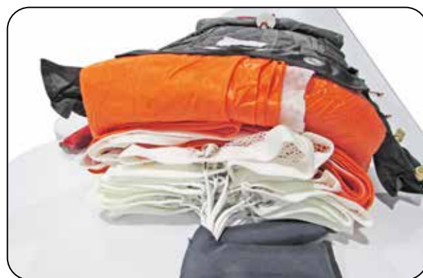
13.2 Folding the canopy into the deployment bag.
