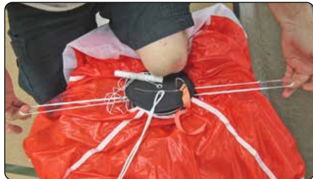
14.14 Compressing the pilot chute.
