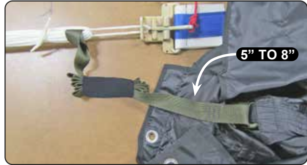
11.2 Stowing the deployment bag bridle.
