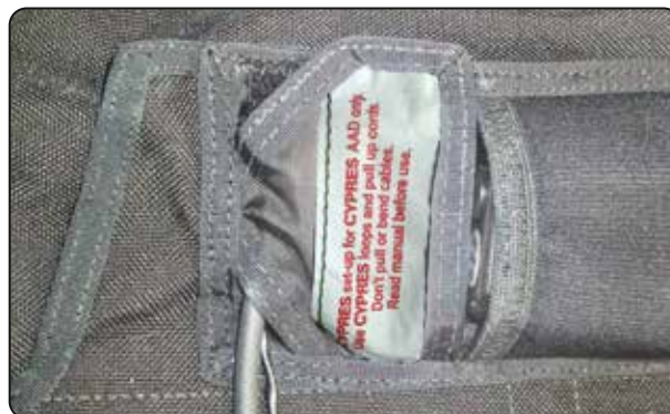
7.2.10 Stowing the excess cable/wire.
