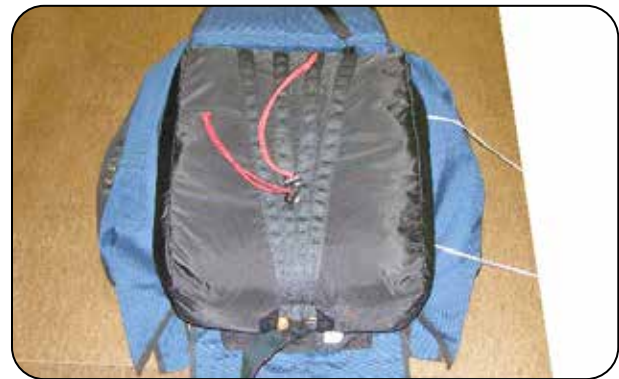
14.1 Placing the bag on the pack tray.
