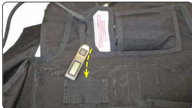
7.2.2 Routing the control unit.
