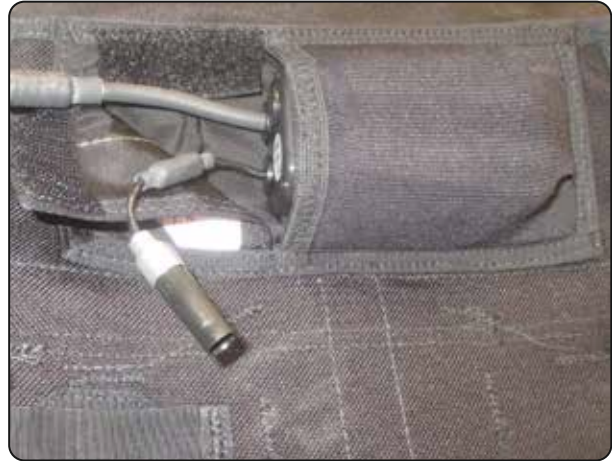
7.2.1 Inserting the CYPRES processor.
