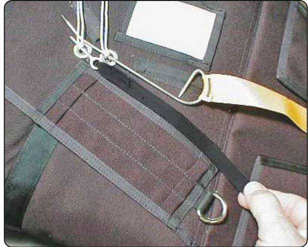
15.2 Stowing the static line.
