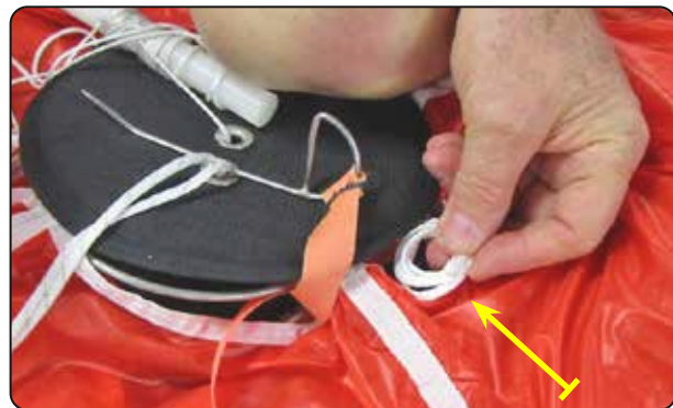
14.15 Clearing the center lines.
