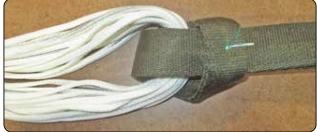
10.2.1 Attaching the deployment bag bridle.
