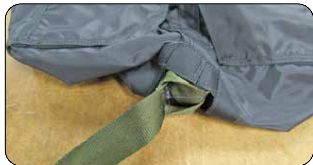
10.2.4 Installing the pilot chute bridle.
