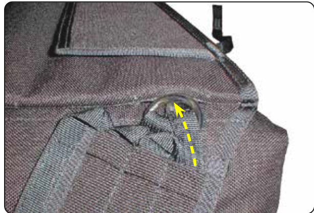
15.4 Stowing the static line.
