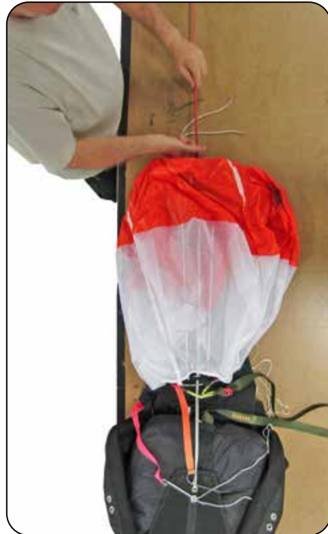
14.13 Threading the pull-up cords through the pilot chute.
