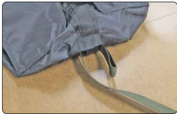
10.2.3 Installing the deployment bag bridle.
