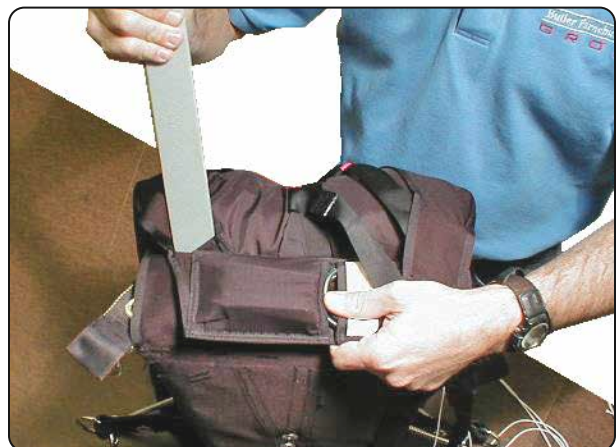
14.20 Dressing the container.
