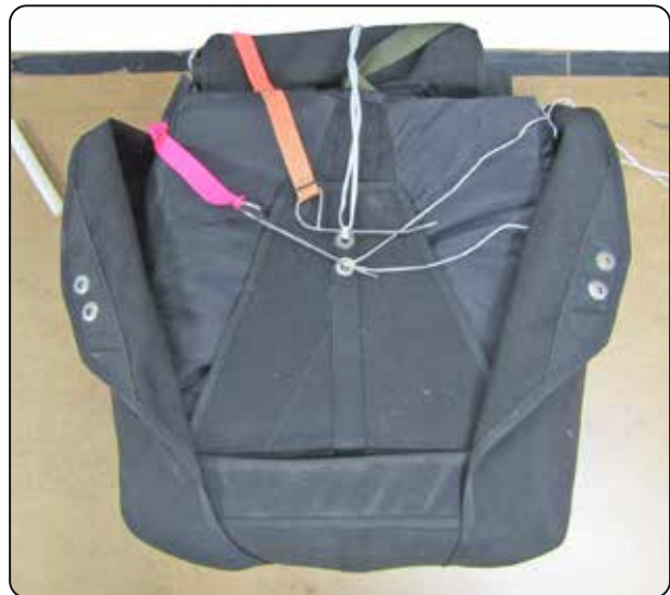
14.12 Closing the bottom flap.
