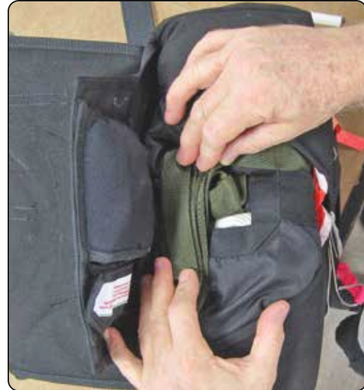
14.21 Stowing the pilot chute bridal.
