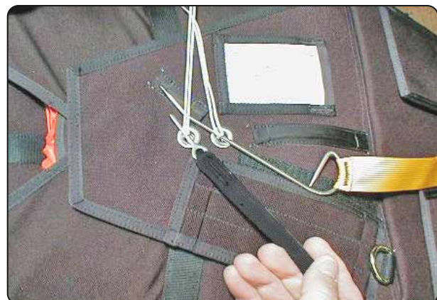
15.1 Seating the static line pin.
