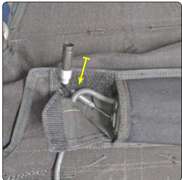
7.2.5 Routing the cutter wire.
