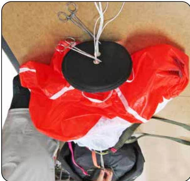
14.13 Threading the pull-up cords through the pilot chute.
