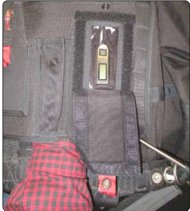
7.2.4 Seating the control unit.
