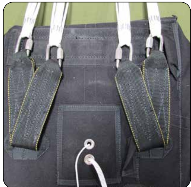
8.4 Attaching the canopy to the container.
