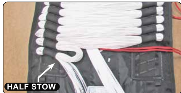
13.5 Stowing the suspension lines.
