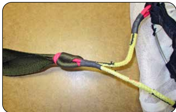
9.2.6 Attaching the pilot chute.
