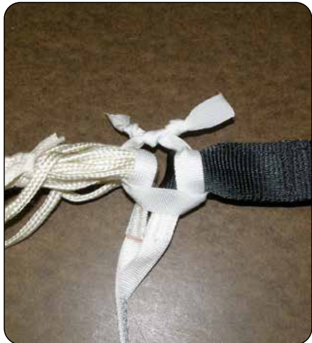
10.1.4 Installing the break tape.
