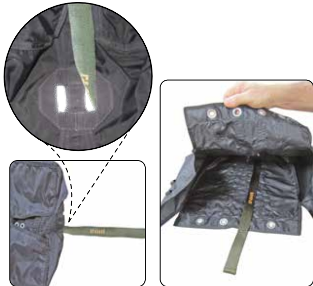
10.2.2 Routing the pilot chute bridle.
