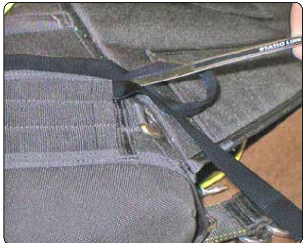
15.3 Stowing the static line.
