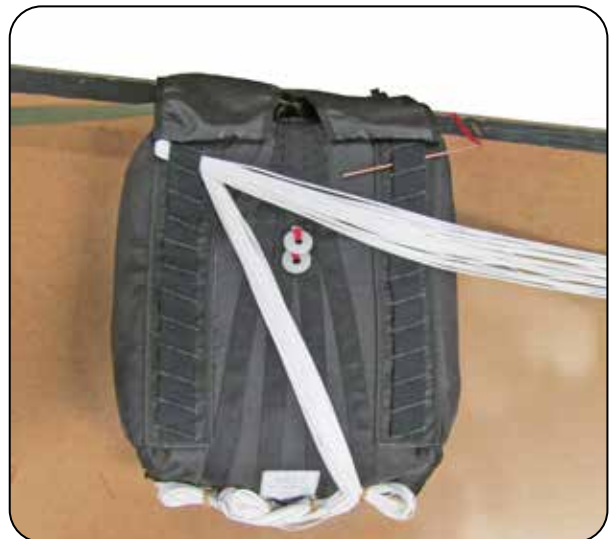
13.4 Stowing the suspension lines.
