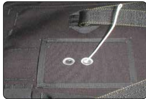
7.3.1 Installing the CYPRES closing loop.
