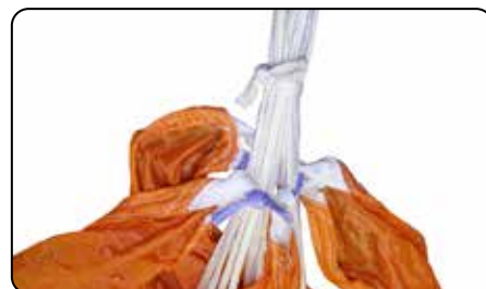
9.2.3 Tying the top tie-tabs.
