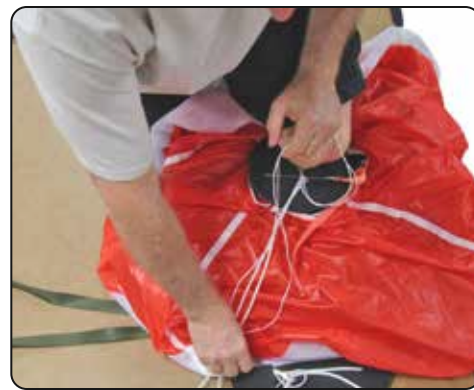
14.14 Compressing the pilot chute.
