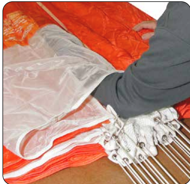
12.3 Stowing the slider.
