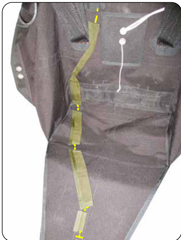
7.2.9 Installing the cutter cable wire.
