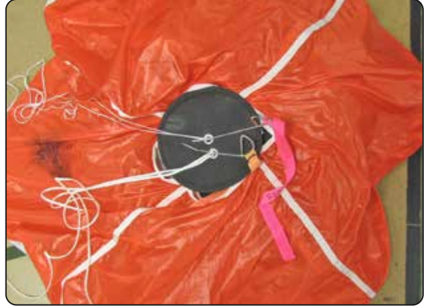
14.16 Pinning the container closing loop.
