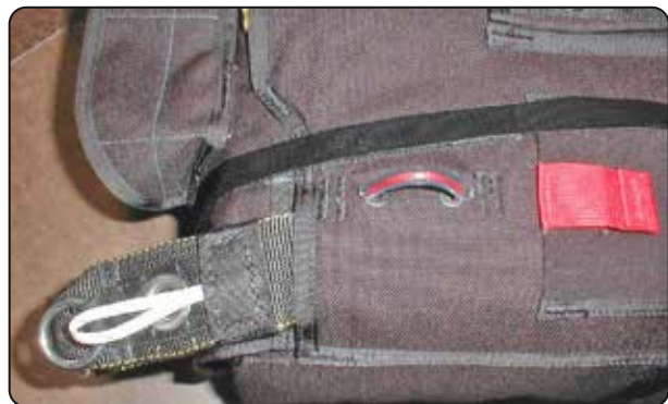
15.6 Stowing the static line.
