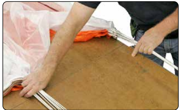
8.2 a. Spreading the main line groups.
