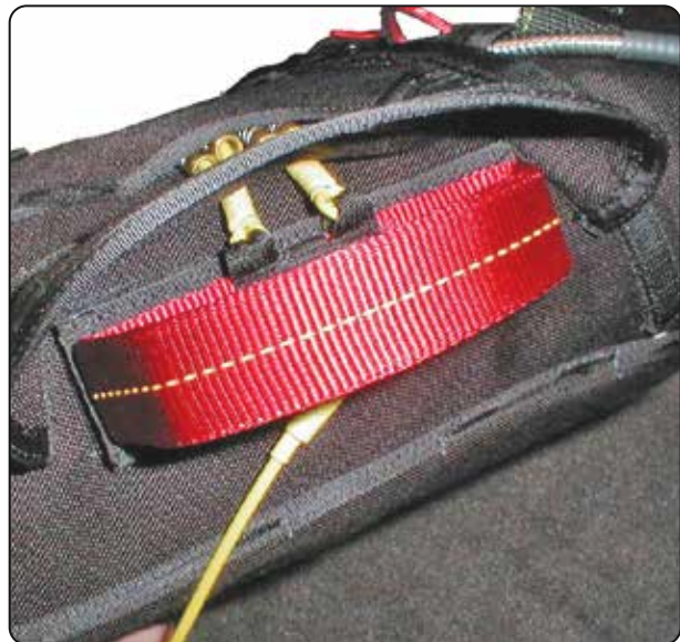
13.1 Installing the release handle.
