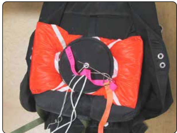
14.17 Folding the pilot chute material.
