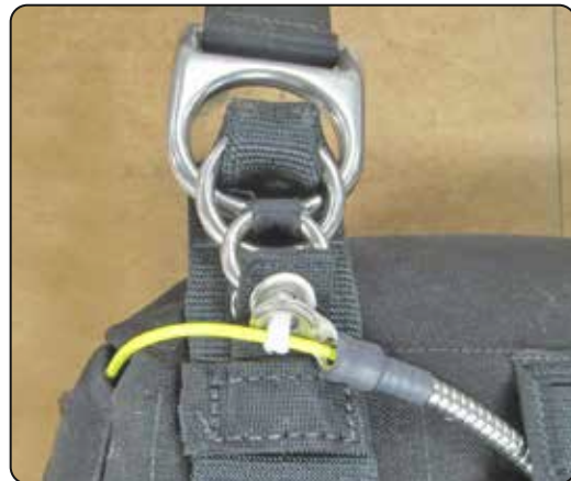
18.2.1 Installing the side attachments.
