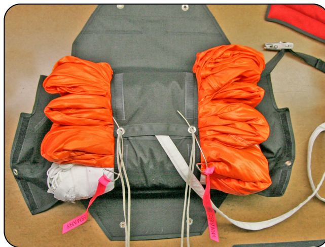
9.8 Closing the top staging flap.
