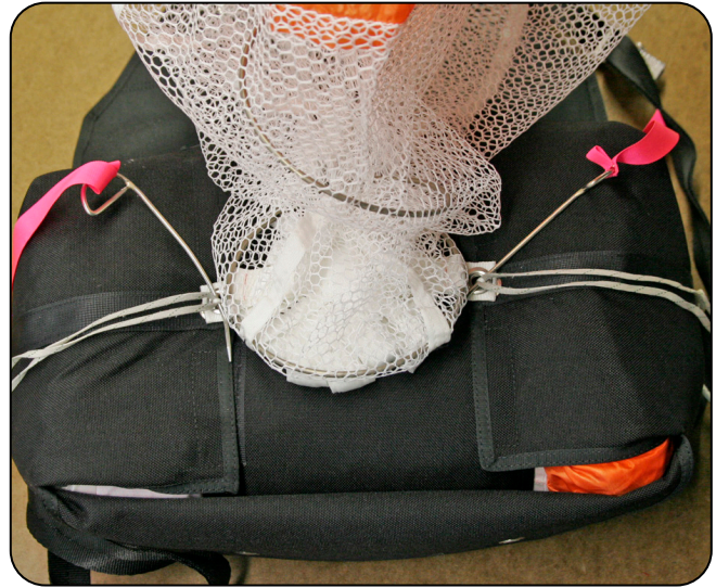
9.12 Stowing the pilot chute.
