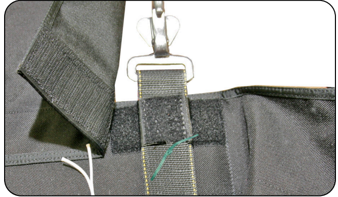
7.2.1 Tacking the riser to the pack tray.
