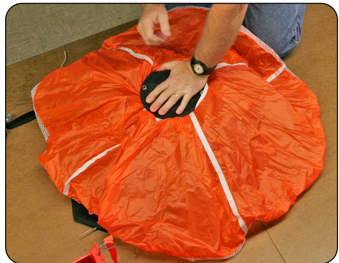
9.13 Compressing the pilot chute.
