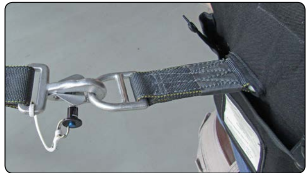
5.1 Attaching the tether to the harness.
