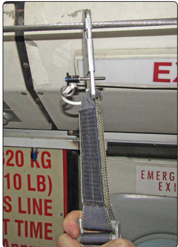
5.2 Attaching the tether to the aircraft.
