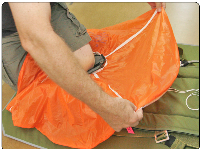
7.15 Compressing the pilot chute.
