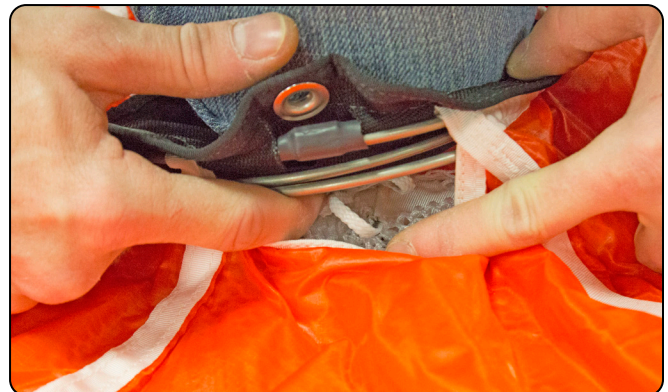
7.17 Folding and stowing the center line.
