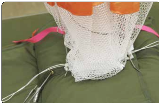
7.14 Setting the pilot chute.
