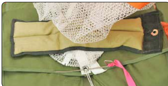
7.13 Stowing the pilot chute bridle.
