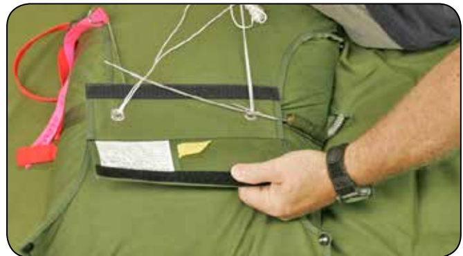
7.23 Closing the right container flap.
