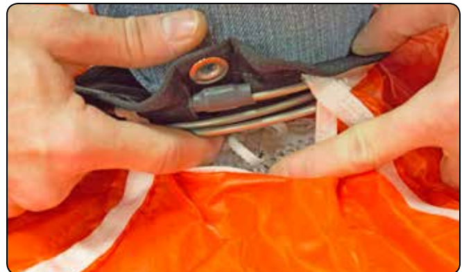
7.17 Folding and stowing the center line.
