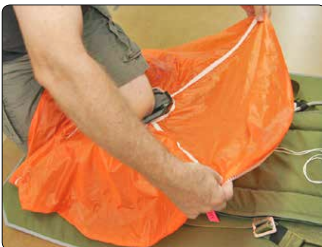
7.15 Compressing the pilot chute.
