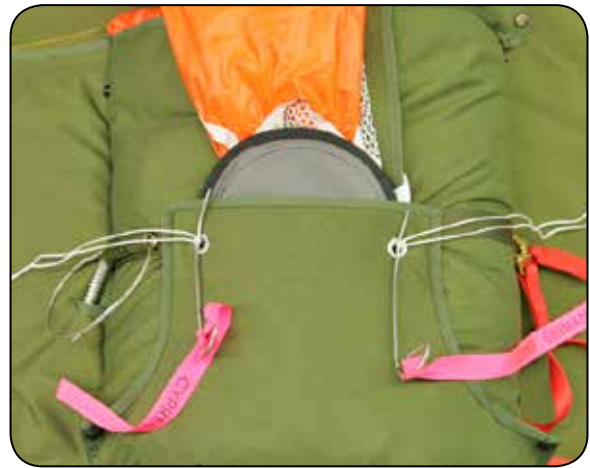
7.22 Closing the left container flap.
