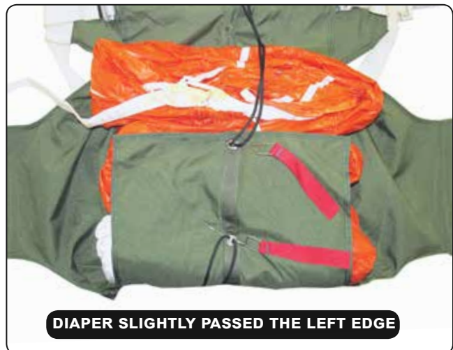
7.11 Closing the bottom flap.
