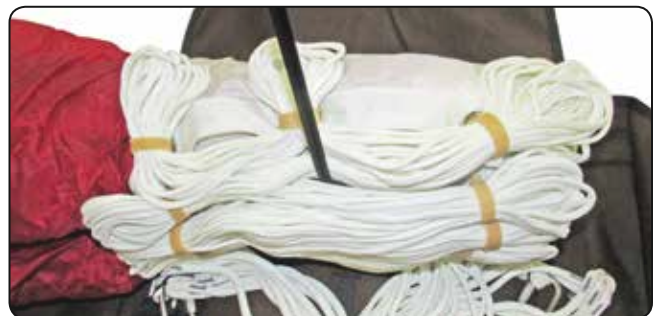
7.8 Routing the closing loop behind the suspension lines.
