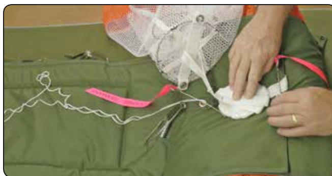
7.13 Stowing the pilot chute bridle.
