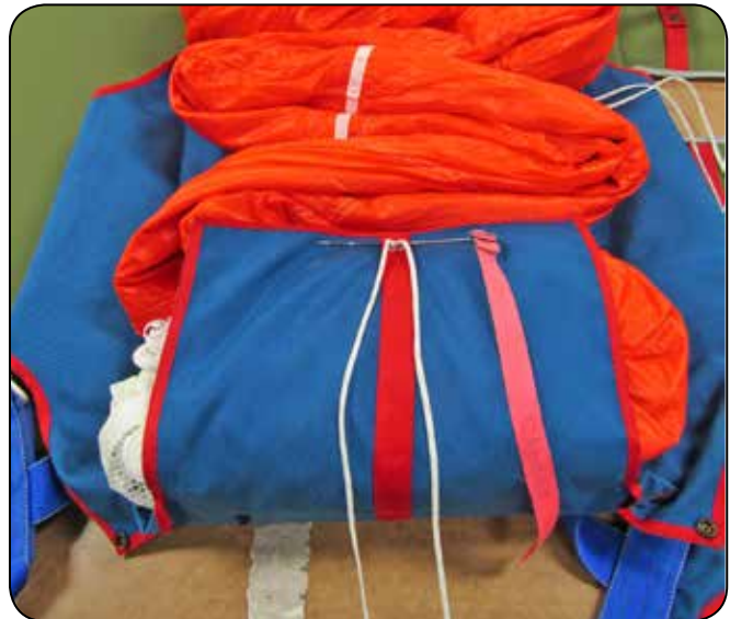
7.6 Closing the bottom flap.
