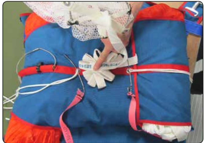
7.9 Stowing the pilot chute bridle.
