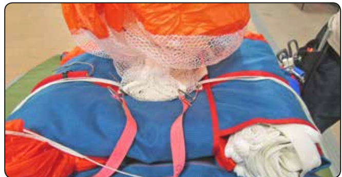
7.10 Setting the pilot chute.
