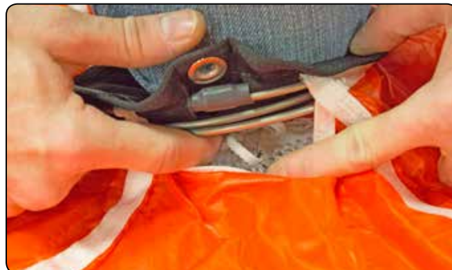
7.13 Folding and stowing the center line.
