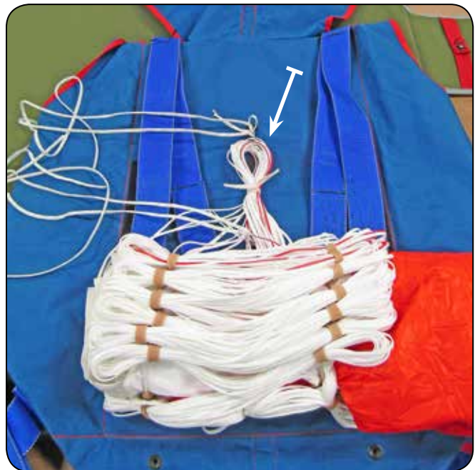
7.4 Tacking the risers.
