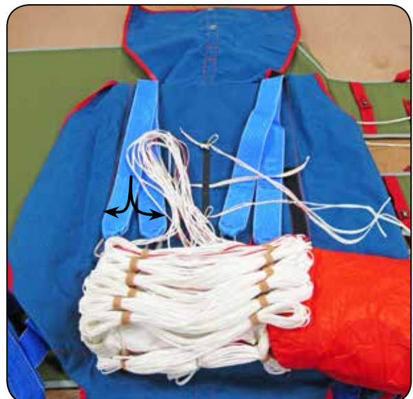
7.2 Placing the diaper.
