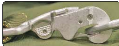
Push the gate down until it is seated over the bearing.
