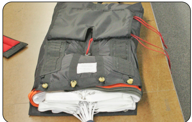
6.1.4 Folding the canopy into the deployment bag.
