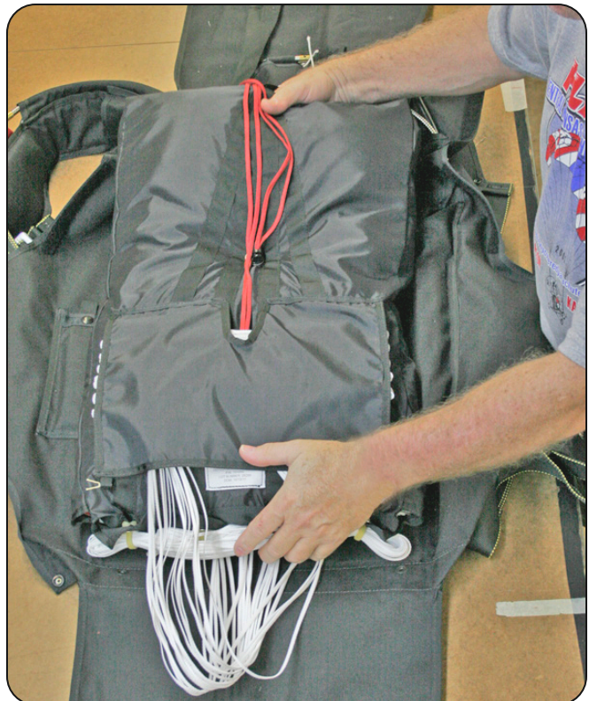
6.3.1 Placing the bag.
