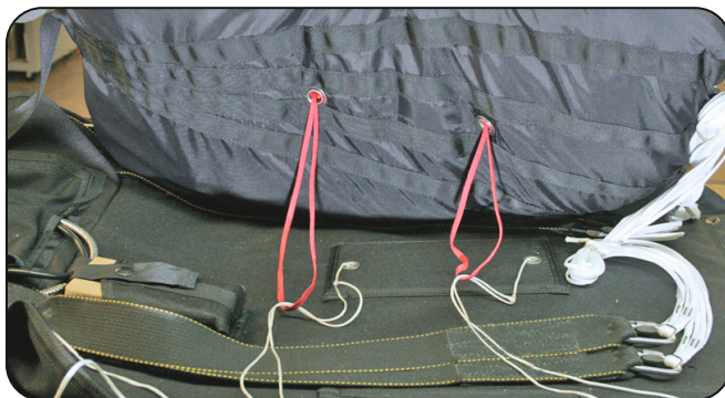
6.3.5 Threading the pull-up cords.
