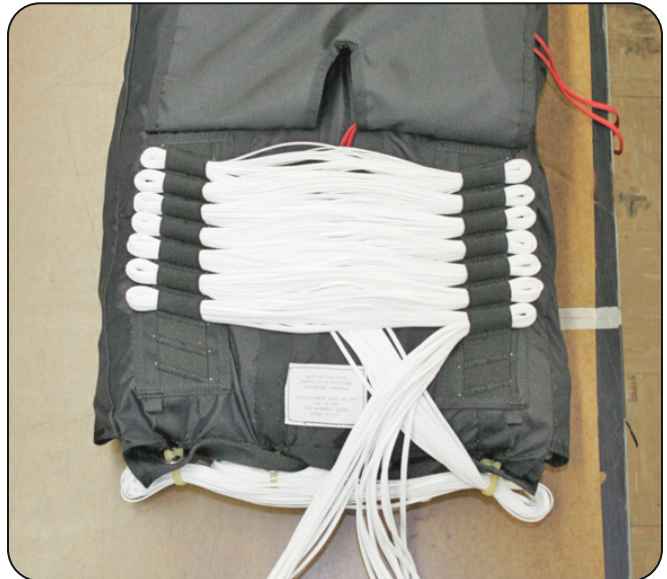
6.2.3 Stowing the suspension lines.
