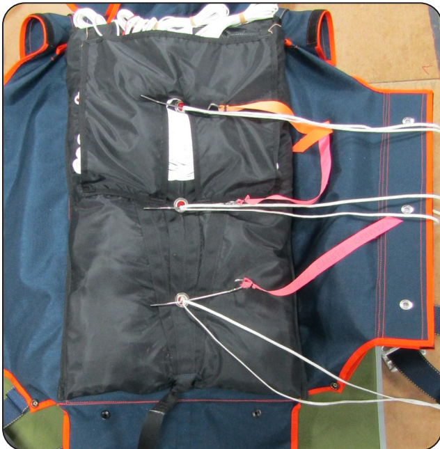
7.3.5 Securing the pull-up cords.
