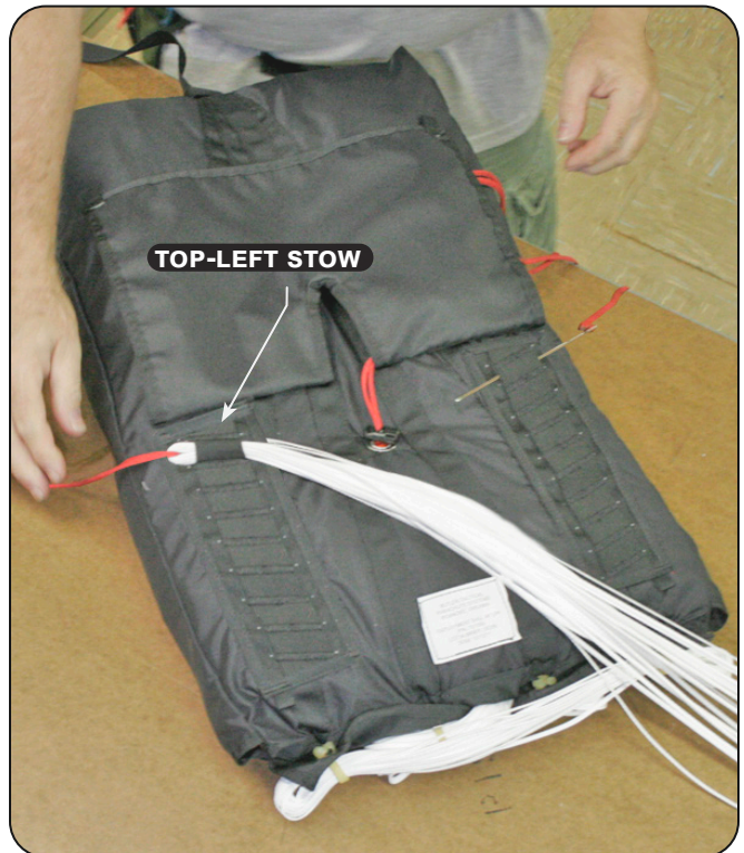
6.2.2 Stowing the suspension lines.
