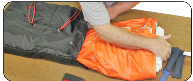
6.1.3 Folding the canopy into the deployment bag.
