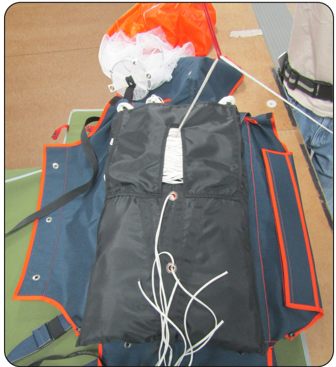
7.3.4 Threading the pull-up cords.
