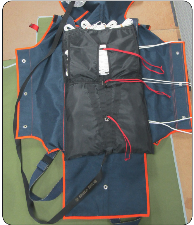
7.3.3 Placing the bag into the container.
