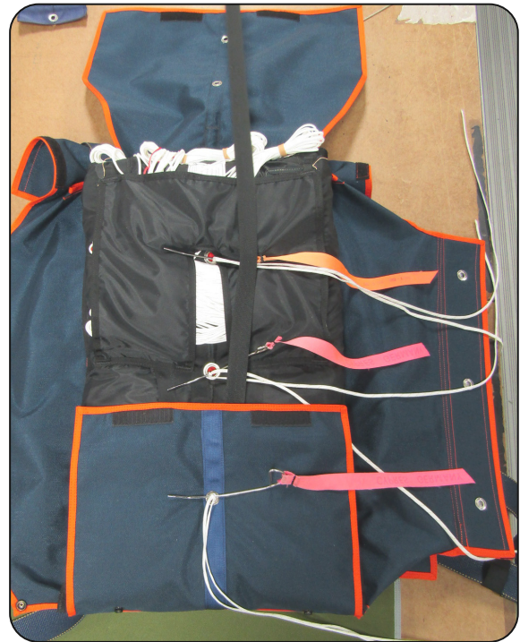
7.3.6 Closing the bottom flap.
