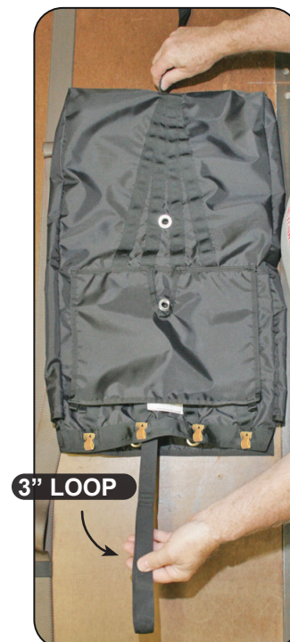
5.8 Pilot chute bridle through the deployment bag.
