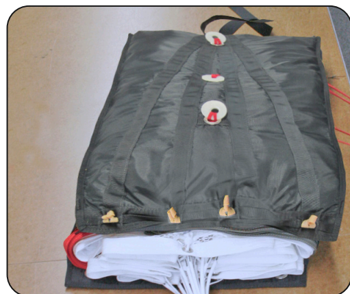
7.1.4 Folding the canopy into the deployment bag.
