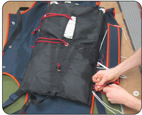
7.3.4 Threading the pull-up cords.
