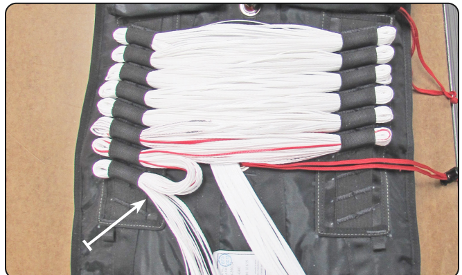
6.2.3 Stowing the suspension lines.
