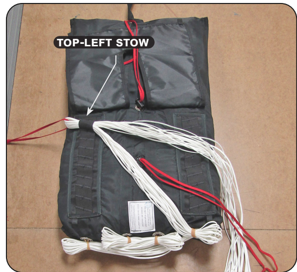
7.2.3 Stowing the suspension lines.
