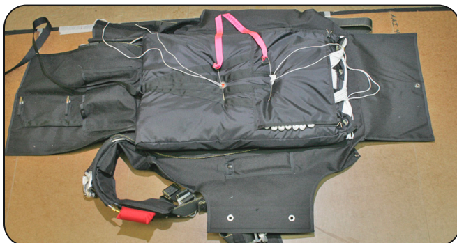
6.3.6 Securing the pull-up cords.
