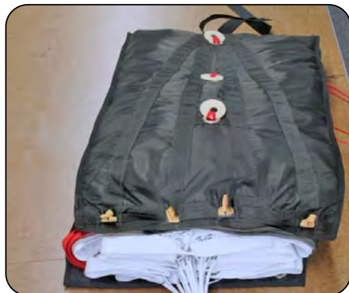
7.1.4 Folding the canopy into the deployment bag.
