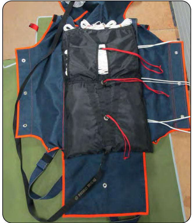
7.3.3 Placing the bag into the container.
