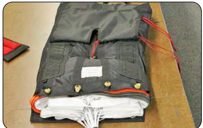
6.1.4 Folding the canopy into the deployment bag.
