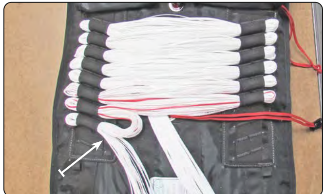
6.2.3 Stowing the suspension lines.
