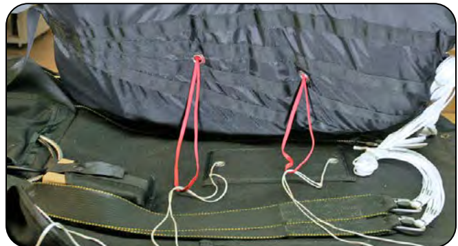
6.3.5 Threading the pull-up cords.
