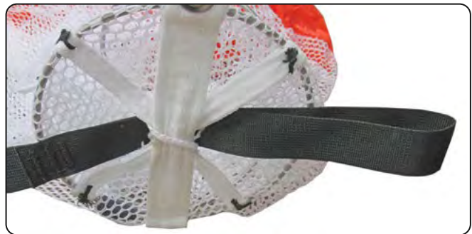
5.12 Threading the bridle.
