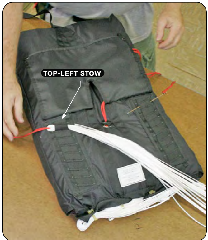
6.2.2 Stowing the suspension lines.
