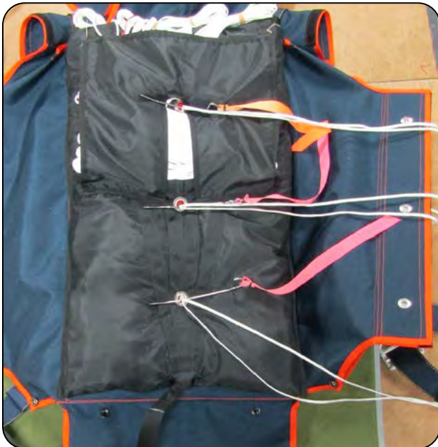
7.3.5 Securing the pull-up cords.
