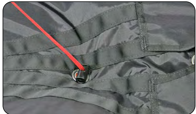
6.1.2 Installing the locking pull-up cord.
