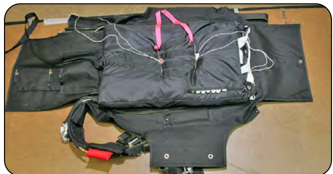
6.3.6 Securing the pull-up cords.
