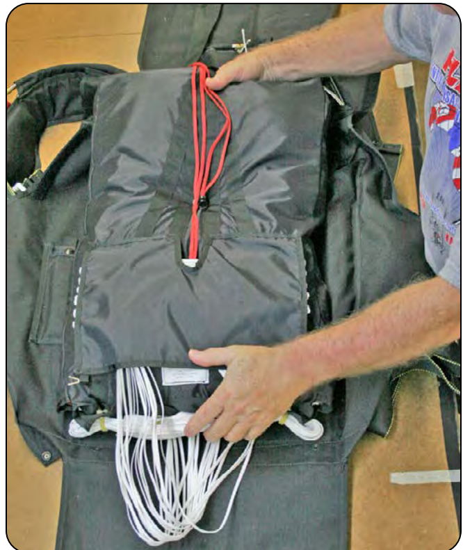
6.3.1 Placing the bag.
