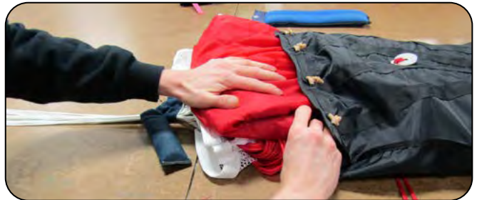
7.1.3 Folding the canopy into the deployment bag.
