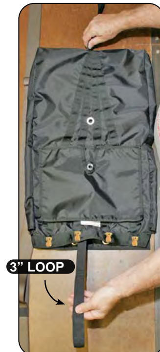
5.8 Pilot chute bridle through the deployment bag.
