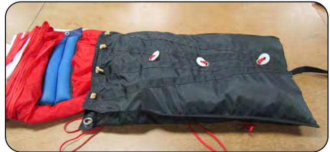
7.1.3 Folding the canopy into the deployment bag.
