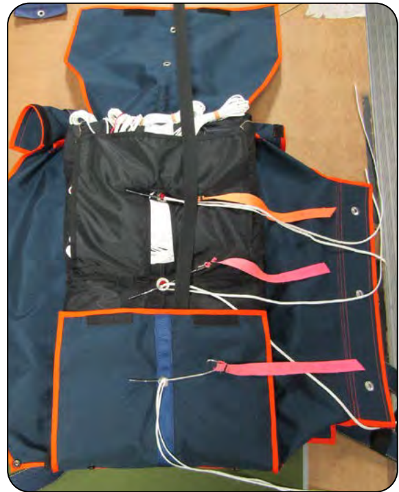
7.3.6 Closing the bottom flap.
