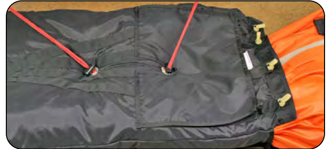
6.1.3 Folding the canopy into the deployment bag.
