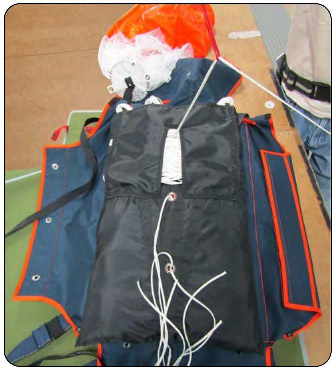
7.3.4 Threading the pull-up cords.
