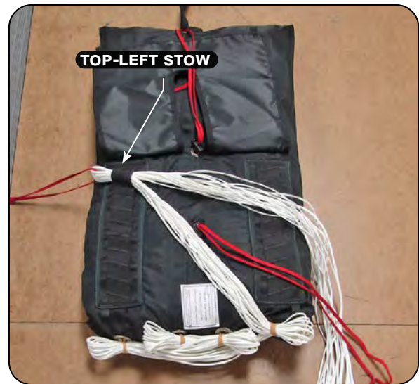
7.2.3 Stowing the suspension lines.
