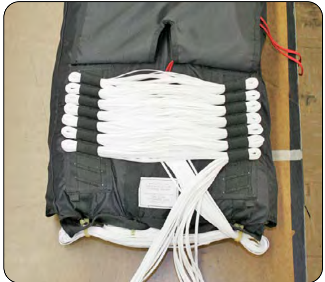
6.2.3 Stowing the suspension lines.
