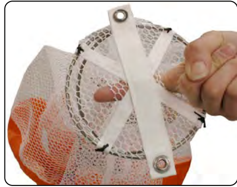
5.11 Cutting the pilot chute mesh.
