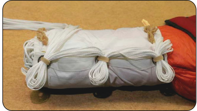
10.6 Closing the remaining locking stows.
