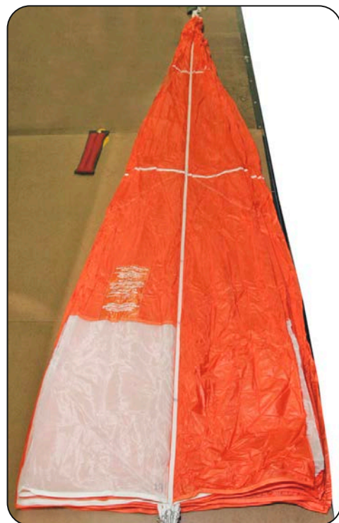
9.2 Flaking the canopy.
