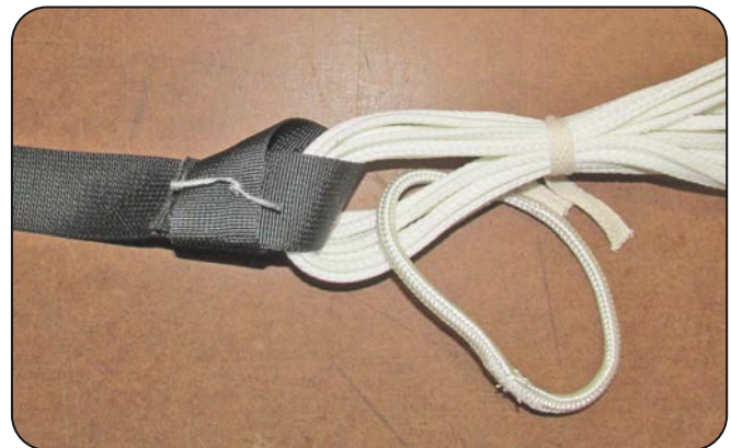
8.1 Bridle installation onto the apex.
