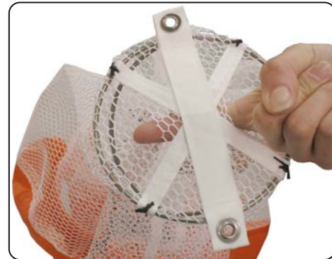
7.4 Cutting the pilot chute mesh.
