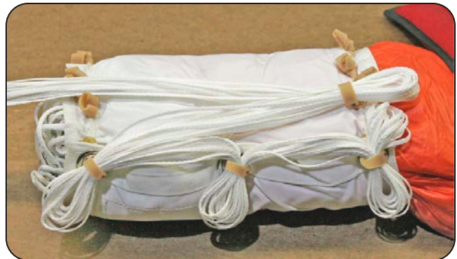
10.6 Closing the remaining locking stows.
