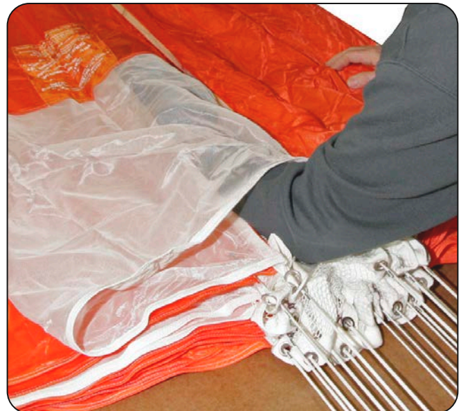
9.3 Stowing the slider.
