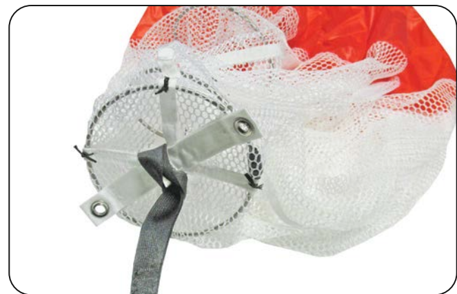
8.4 Installing the pilot chute.
