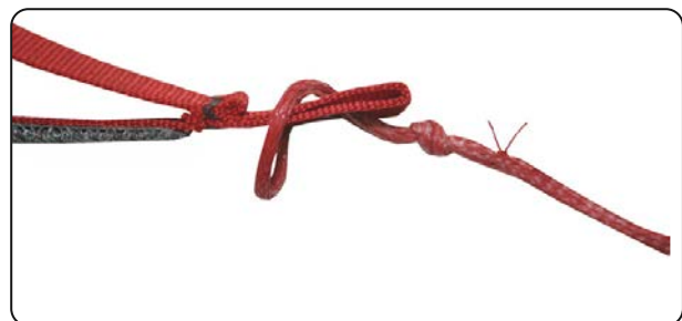
6.5 Installing the steering line toggle.
