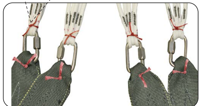
6.1 Tacking the risers.
