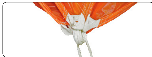
7.11 Tying the top tie-tabs.
