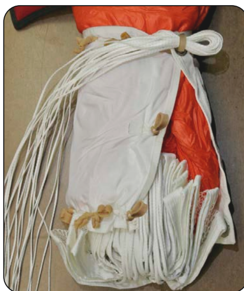
10.4 Closing the first locking stow.
