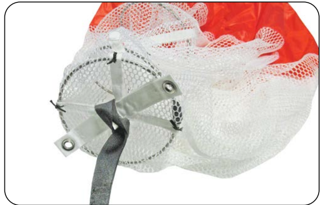
7.6 Installing the pilot chute.
