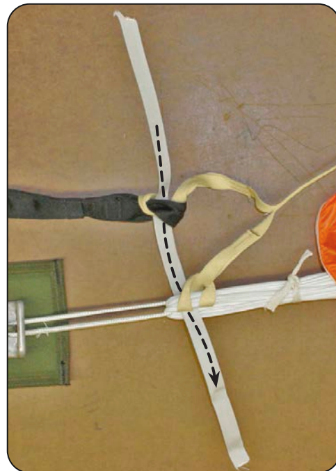
7.6 Installing the pilot chute.
