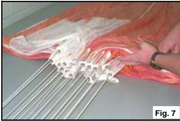
Figures 7 & 8. After inserting the slider into the main canopy, flake each gore of the slider into the corresponding gore of the canopy.
