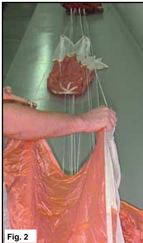
Figure 2. Perform a continuity check to ensure proper routing of the suspension lines through the slider and rotation on the connector links.
