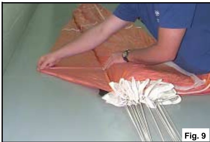
Figures 9 & 10. At the rigger's discretion, the gores may be folded 90 degrees (parallel to the radial seam) as a group or individually.
