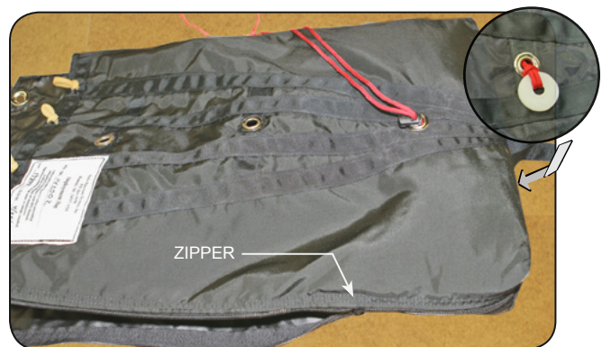
7.4 Installing the locking pull-up cord.
