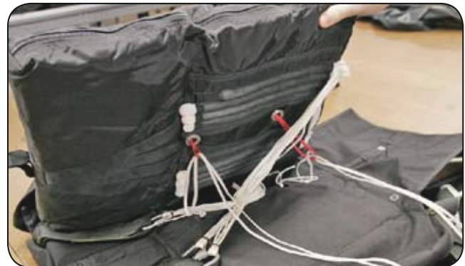
9.4 Threading the pull-up cords.
