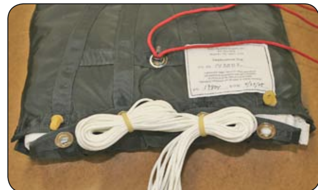
8.1 Closing the inside locking stows.
