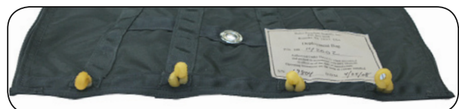
6.3 Installing the locking stow bands.
