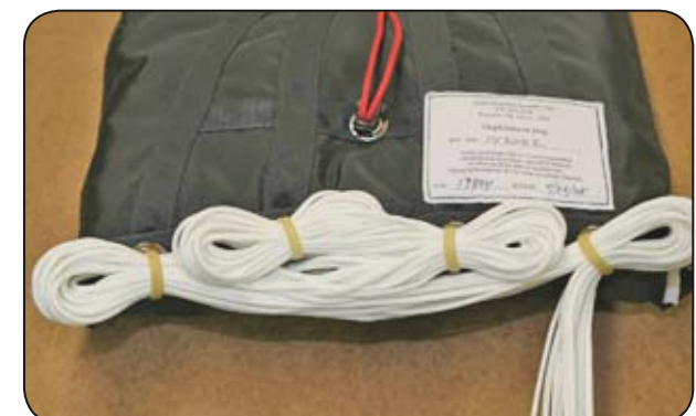
8.2 Closing the outside locking stows.
