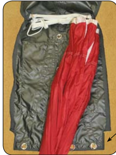
7.2 Stowing the incremental bridle.
