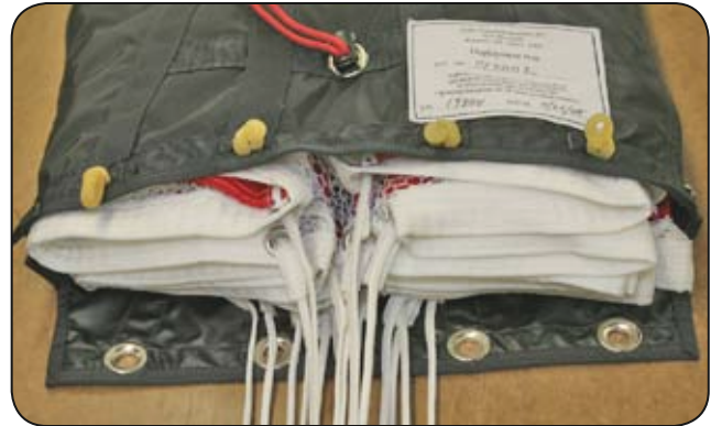
7.7 Filling the front of the bag.
