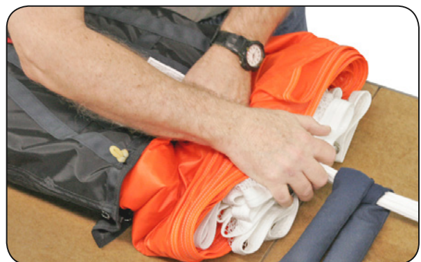
7.6 Inserting the skirt of the canopy.
