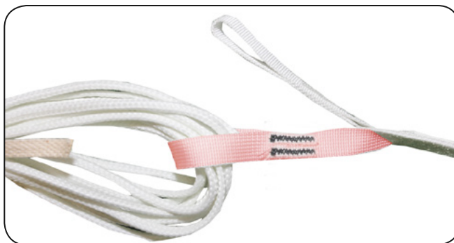
6.4 Sewing the incremental bridle to the apex.
